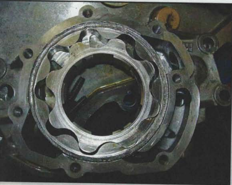
A front mounted oil pump may be damaged if it is not centered correctly on the crankshaft.
