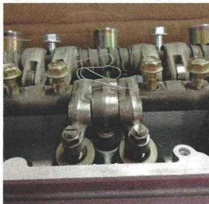
can easily fall out and be lost once the rocker panel is removed from the cylinder head. Before removing the panel, use a small wire to hold the three rockers together.
