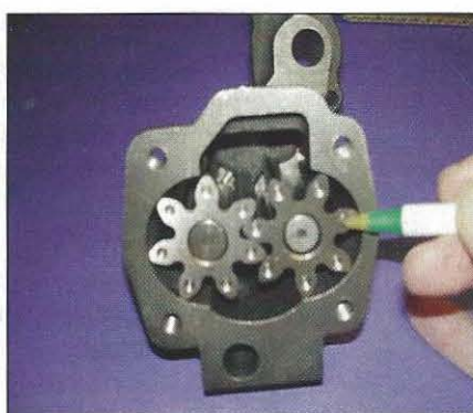
A slightly out of focus shot showing how small dimples have been machined into the ends of the gear teeth to reduce cover and housing wear in a SB Chevy oil pump.
