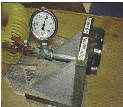
Schumann says his new oil pump test stand allows engine builders to not only test and verify pump flow across a wide range of speeds, but to also check the pump's relief pressure.
