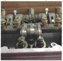
can easily fall out and be lost once the rocker panel is removed from the cylinder head. Before removing the panel, use a small wire to hold the three rockers together.
