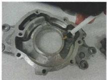
the result of what happens when the oil pump lacks sufficient clearance because of a stack up of manufacturing tolerances when a spacer is used. The thrust surface of the housing and the inner drive gear both have turned black from the excessive friction and heat. Steel turns black at 800 to 900 degrees F, and blue at 1,050 to 1,100 degrees F. The thrust surface in the pump housing has also been worn down nearly .014".
