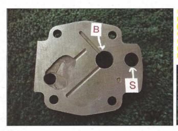
Schumann's new "Dual Feed" oil pump for Chevy small block circle track applications is a "wet pump with a dry sump attitude," according to the company's leader. The new pump has a second side inlet port that allows the pump to maintain oil flow at high rpm (inside of cover shown at left). The pump uses a spring-loaded steel check ball to control internal oil pressure instead of a cup valve (below). The check valve design won't jam or stick like a cup valve can if the pump sucks in any debris.
