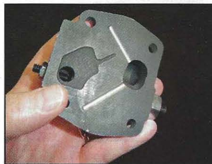
Bottom side of oil pump with an adjustable pressure relief valve.
