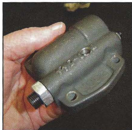
The spring loaded relief valve opens when the oil pressure reaches its limit.
